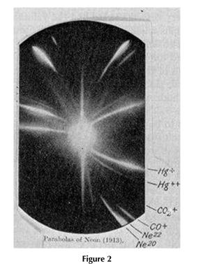
**THOMSON'S PHOTOGRAPHS OF NEON ISOTOPES** This photographic plate, from one of J.J. Thomson's experiments, shows two different positions for neon ions, which are now known as the isotopes neon-20 and neon-22.
