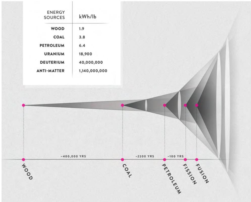
*This progression of cones of increasing pitch show the natural progression of sources of fuels of higher energy density. Apexes represent the time of their discovery. As a new cone reaches the previous one, the old technology becomes eclipsed in its use in the economy. Both the rate of discovery, and the relative energy ratios are increasing dramatically. Deuterium is used here as the fuel for fusion reactions.*
