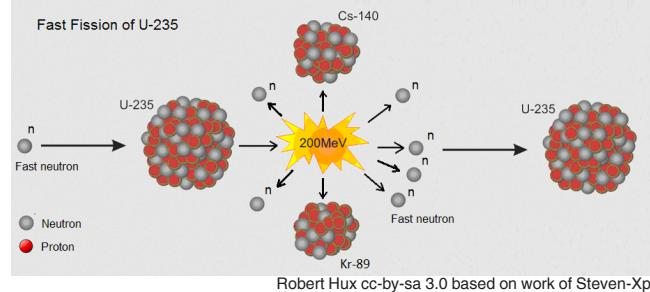
Figure 5. Fast nuclear fission of U-235 producing two typical fission products.
