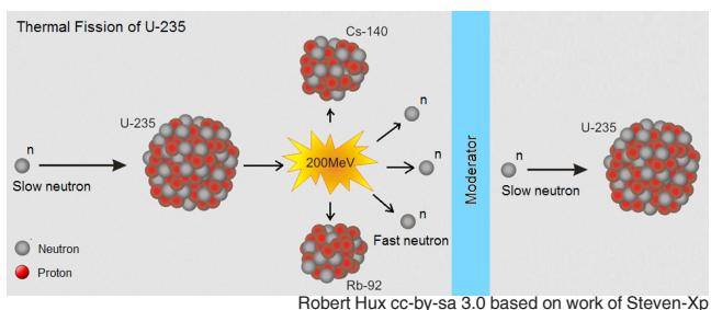
Figure 3. Thermal nuclear fission of U-235 initiated by the capture of a slow neutron produces two smaller atoms (Rb-92 and Cs-140 shown here only one possibility among many) and an average of 2-3 fast neutrons, which can be slowed down by interaction with a moderator (water, heavy water or graphite) to increase probability of capture by another U-235 nucleus and initiate a chain reaction.
