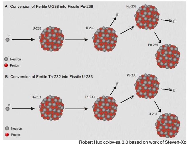
*Figure 6. The real potential of nuclear fission depends on the use of fast reactors to efficiently create new fissile materials, through two paths: A. Conversion of the non-fissile uranium (U-238) into fissile Pu-239. B. Conversion of the more abundant thorium (Th-232) into fissile U-233.*
