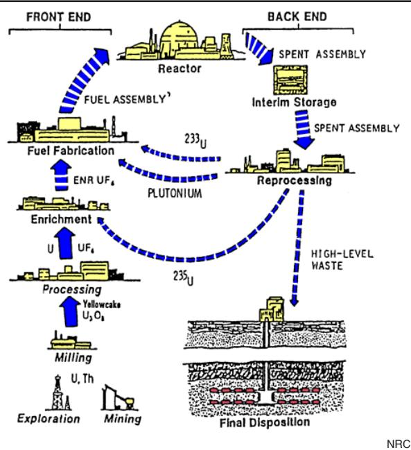
Figure 4. The closed nuclear fuel cycle of existing nuclear reactors.
