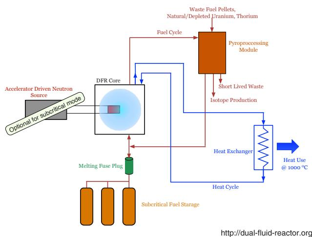
Figure 2. DFR fuel and cooling loops. The pyro-processing module prepares the molten salt fuel which is pumped into the DFR core, and continuously extracts and separates useful isotopes from short term waste. Molten lead carries the heat from the DFR core and fission products out of the reactor to the heat exchanger. In case of loss of cooling, melting fuse plugs allow the molten salt fuel and the fission products to be drained out of the reactor core, safely shutting the reactor down.
