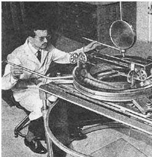
Jacques Bourgeot, laboratory director, operating the Allais paraconical pendulum, photographed by Maurice Allais. He is operating the measuring circle for the pendulum, which allows measurement of the direction of the swing and the two axes of the flat ellipse which the pendulum bob traces out.
